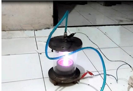
Gambar 4.3b. mekanisme kerja DC Magnetron Sputtering .
