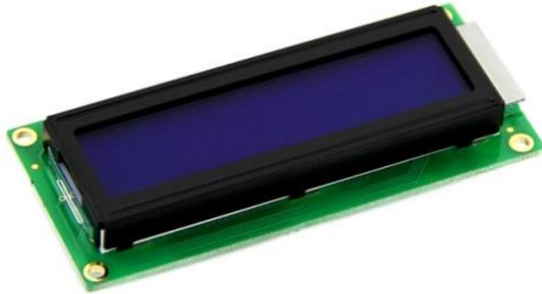
Gambar 2.19 LCD 16 X 2
