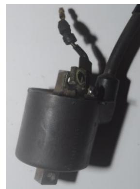
**Gambar 3.7.** Koil (*Ignition Coil*)
