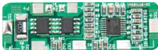
Gambar 2.31. Battery Management System
