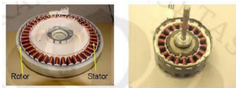
Gambar 2.18 Penampang Motor BLDC (Sumber : Dharmawan, 2009)
