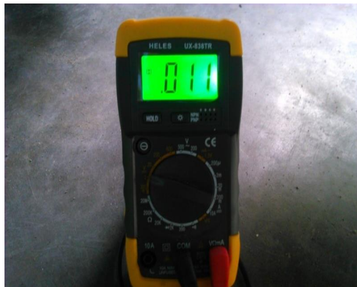
Gambar 4.9 Tegangan pulser saat Rpm 5000
