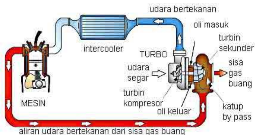
Gambar 2.8 Prinsip Kerja Turbocharger (Sumber : Automotive, 2011)
