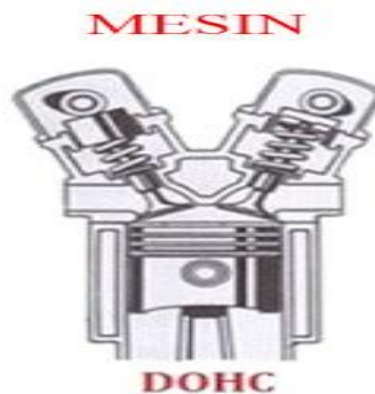
Gambar 2.5 DOHC ( Double Over Head Camshaft ) (Sumber : Teknik otomotif.com, 2015)
