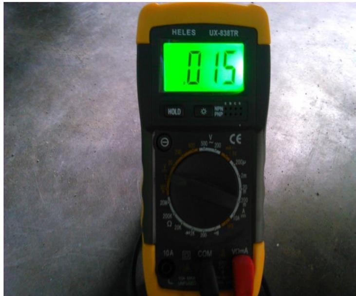
**Gambar 4.10** Tegangan pulser saat Rpm 10.000
