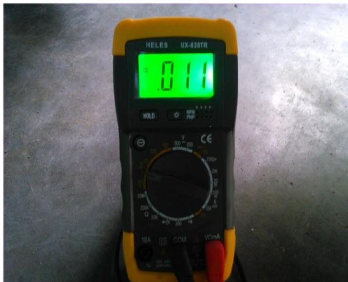
**Gambar 4.9** Tegangan pulser saat Rpm 5000
