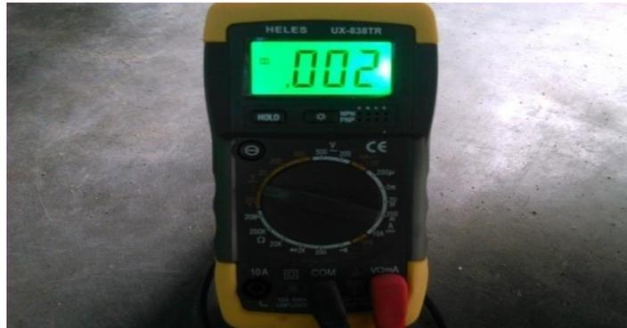
**Gambar 4.8** Tegangan pulser saat Rpm 1500
