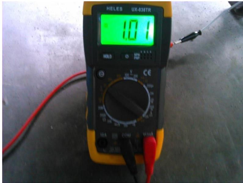
**Gambar 4.11** Tegangan Op-amp saat Rpm 1500
