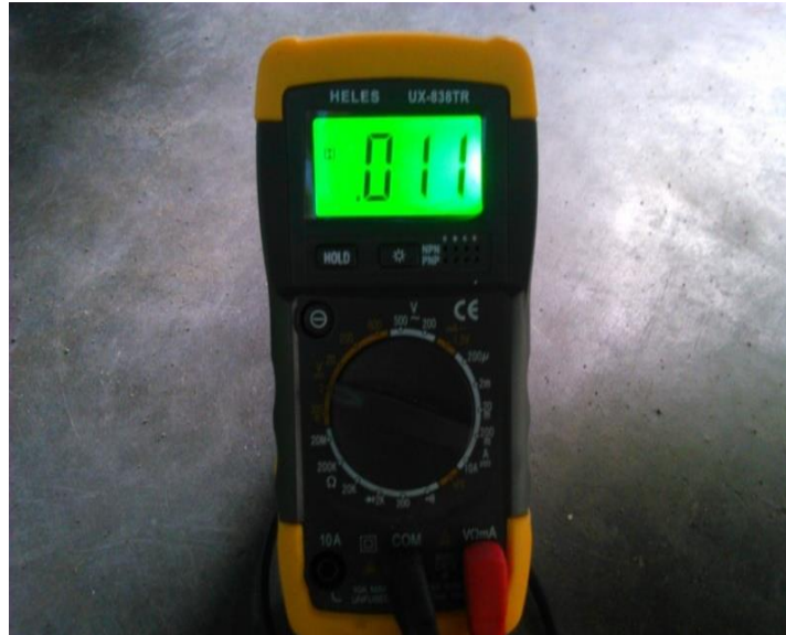
Gambar 4.9 Tegangan pulser saat Rpm 5000
