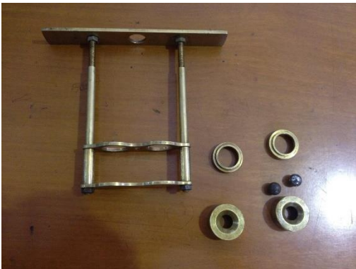
Gambar 17. Alat uji titik lembek ( ring and ball )
