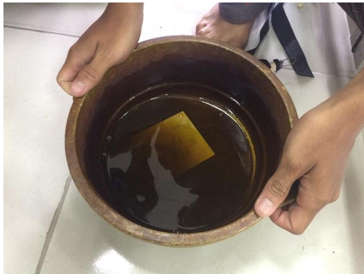
Gambar 3.5 Proses Pelarutan PCB
