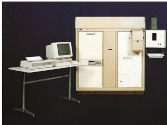
Gambar 3.14 *Spectrometer Type ARL 3560*
