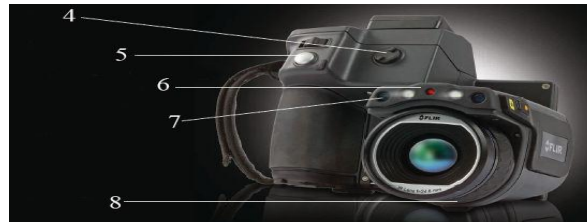
Gambar 2.2 Bagian-bagian kamera Infrared Thermography
