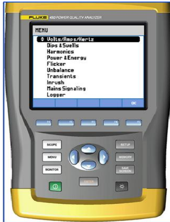
Gambar 2.21 Power Quality Analyzer
