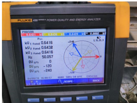
Gambar 4.9 display information Power Quality and Energy Analyzer Fluke series-435.
