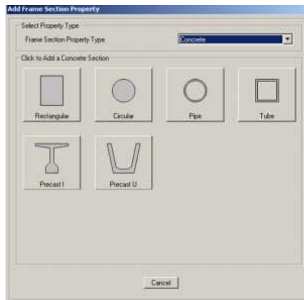
Gambar 3.18 Kotak dialog add frame section property
