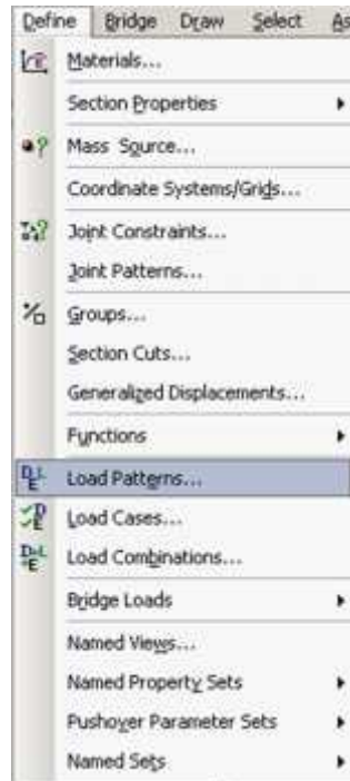
Gambar 3.32 Perintah Define menu > Load patterns
