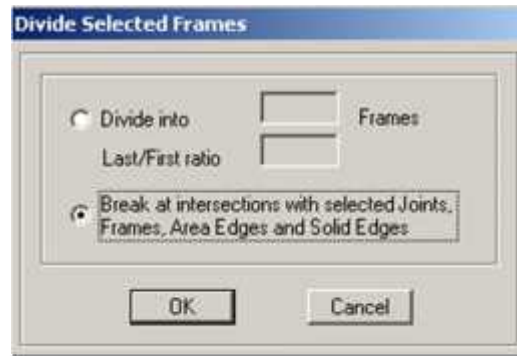
Gambar 3.30 Kotak dialog Divide selected frame
