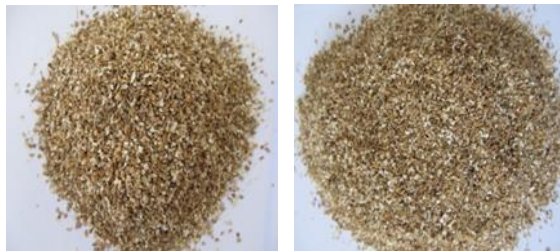
Fig.1. Peanut shell filler: (a) coarse particles, (b) fine particles
