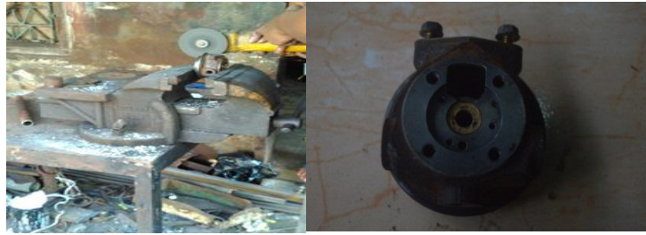
Gambar 4. 4 CHRA ( Center Housing & Rotation Assembly )
