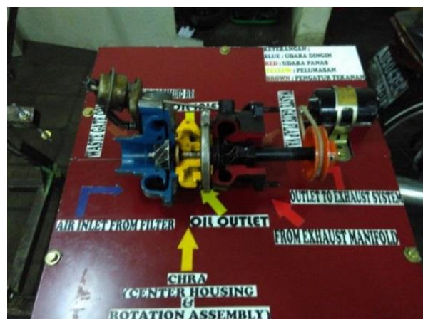
Gambar 4. 8 cara kerja Turbocharger
