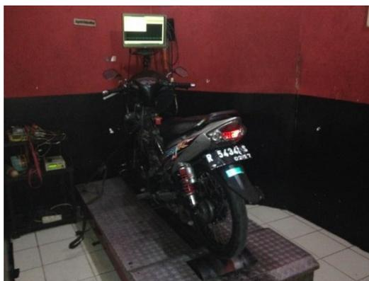
Gambar 5. Dinamometer.
