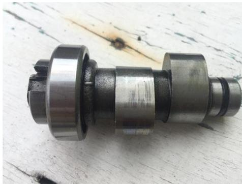
Gambar 1. *Standard Camshaft*.
