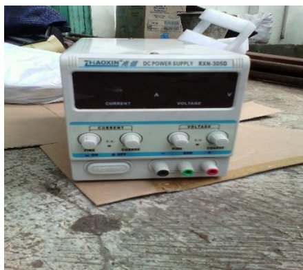
Gambar 3.2 DC Power Supply
