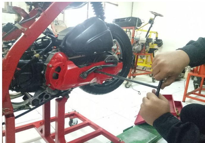
Gambar 3.30 Proses memasang cover CVT
