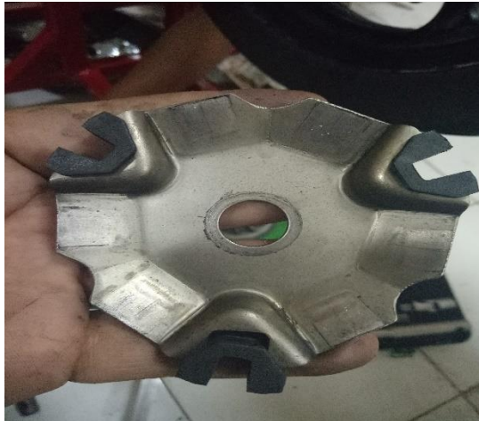
Gambar 3.14 Proses memeriksa ramp plate
