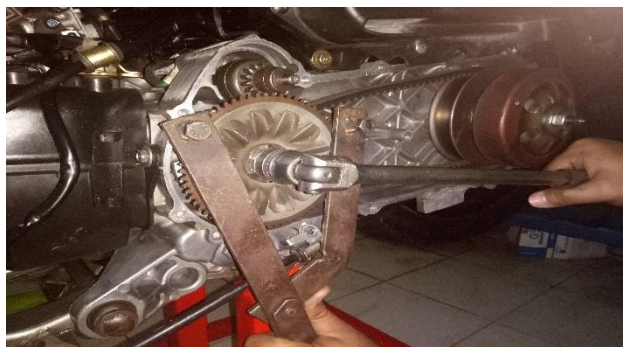
Gambar 3.4 Proses melepas drive pulley face
