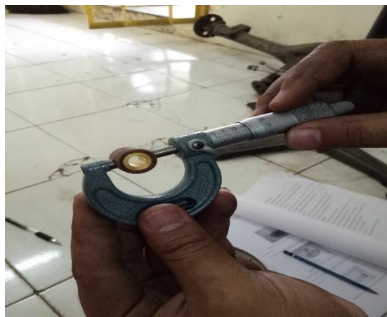
Gambar 3.15 Proses mengukur weight roller
