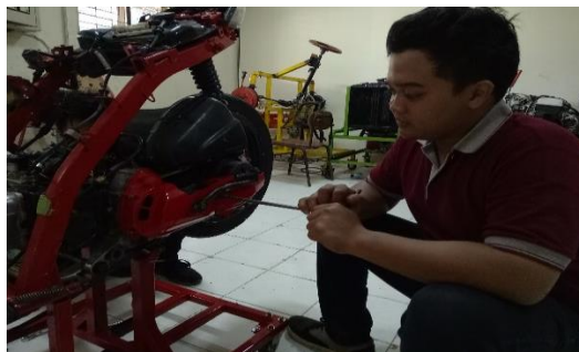
Gambar 3.3 Proses melepas cover CVT
