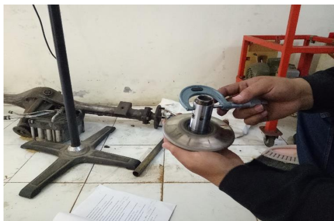
Gambar 3.19 Proses mengukur driven face
