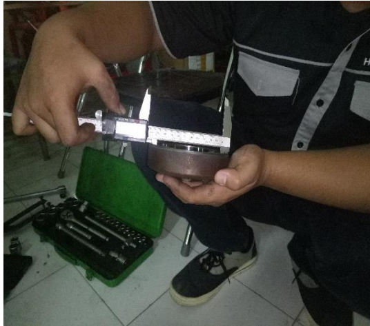
Gambar 3.16 Proses mengukur outer clutch
