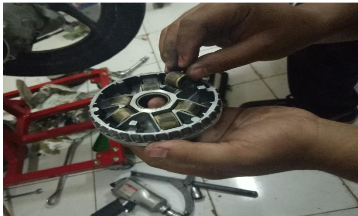
Gambar 3.24 Proses memasang weight roller
