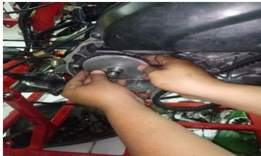
Gambar 3.6 Proses melepas movable drive face
