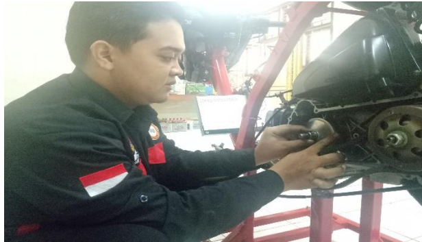
Gambar 3.5 Proses melepas boss movable drive face
