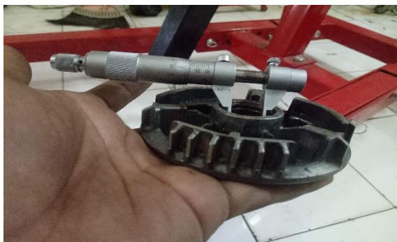
Gambar 3.13 Proses mengukur movable drive face
