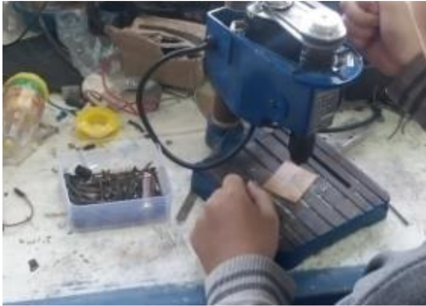
Gambar 3.12 Proses Pengeboran Shield Board .
