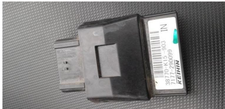
Gambar 2.10 *Electronic Control Module* (PT.Astra Honda Motor : 2014)
