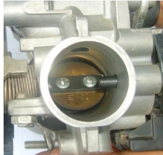
Gambar 2.13 Letak *Intake Air Temperature Sensor* (PT. Astra Honda Motor :2014)
