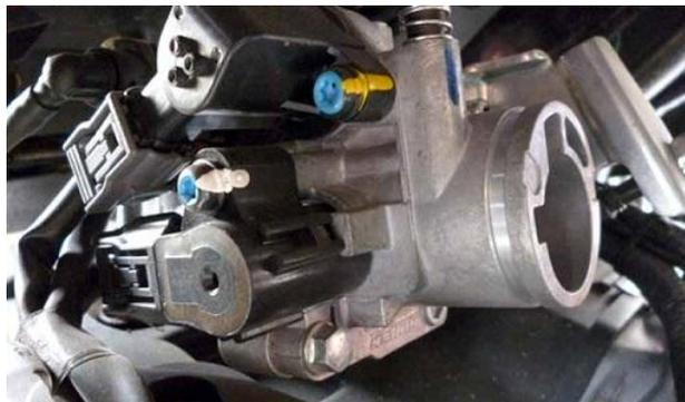
Gambar 2.12 *Throttle Body* (PT. Astra Honda Motor :2014)
