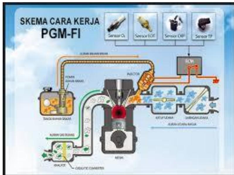
Gambar 2.5 Skema Rangkaian Pompa Bahan Bakar (PT. Astra Honda Motor
