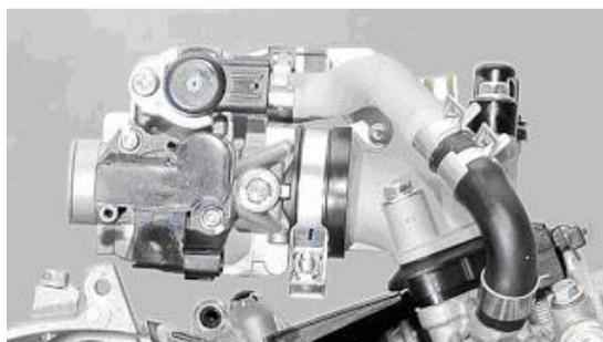
Gambar 2.22 *Idle Speed Control* (PT. Astra Honda Motor :2014)
