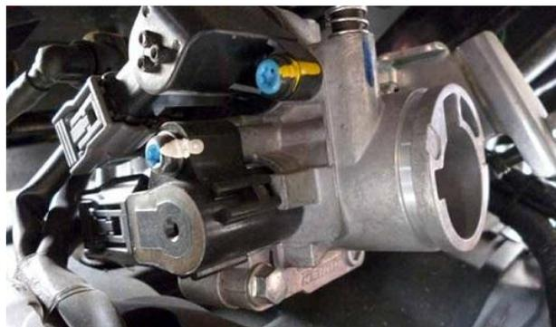
Gambar 2.9 *Throttle body* (PT.Astra Honda Motor : 2014)
