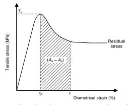
Figure 4. Typical tensile stress–strain curve for toughness index calculation
