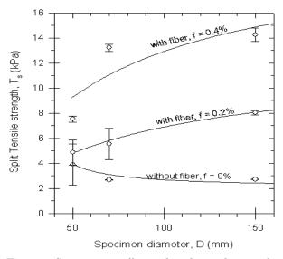
Figure 9. Specimen size effect on the split tensile strength
