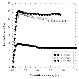
Figure 7. Tensile stress and diametrical strain relationship of the reinforced specimen with 0.4% fiber content
