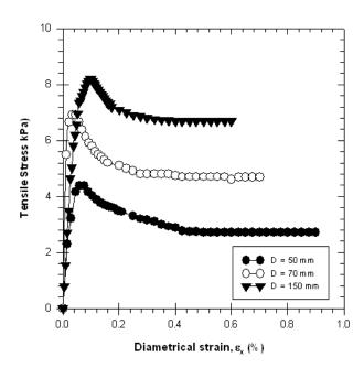
Figure 6. Tensile stress and diametrical strain relationship of the reinforced specimen with 0.2% fiber content
