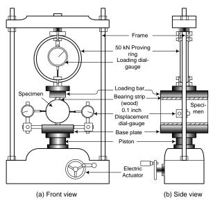
Figure 3. Schematic of test setup
