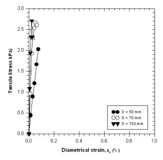
Figure 5. Tensile stress and diametrical strain relationship of the unreinforced specimens
