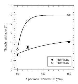
Figure 8. Toughness index of the reinforced soil mixtures
