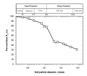
Figure 1. Particle size distribution of the soil used
