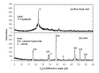
Figure 2. X-Ray diffraction of the rice husk ash and lime
