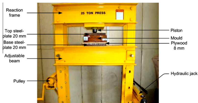
Fig. 3. The design of compressed-hydraulic machine.
