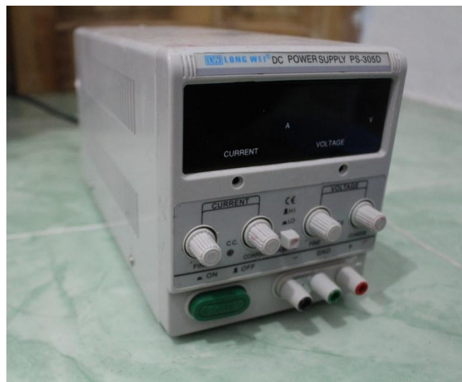
Gambar 3.2. DC Power Supply
