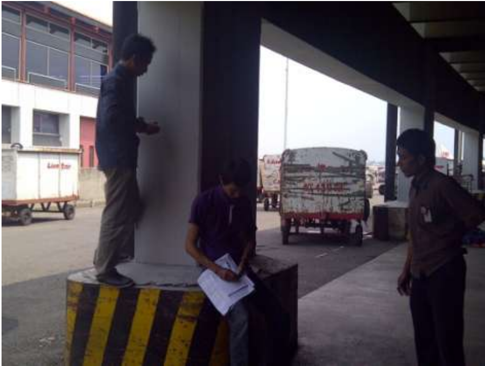
N. UJI HAMMER TEST TERMINAL 1B VIP ROOM
