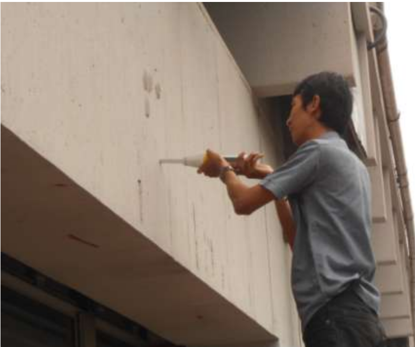
G. UJI HAMMER TEST TERMINAL 1C SHOPPING ARCADE SEBELAH KIRI AREA BREAKDOWN
