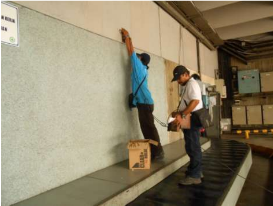
L. UJI HAMMER TEST TERMINAL 1C SHOPPING ARCADE SEBELAH KANAN AREA BAGAGE CLAIM
