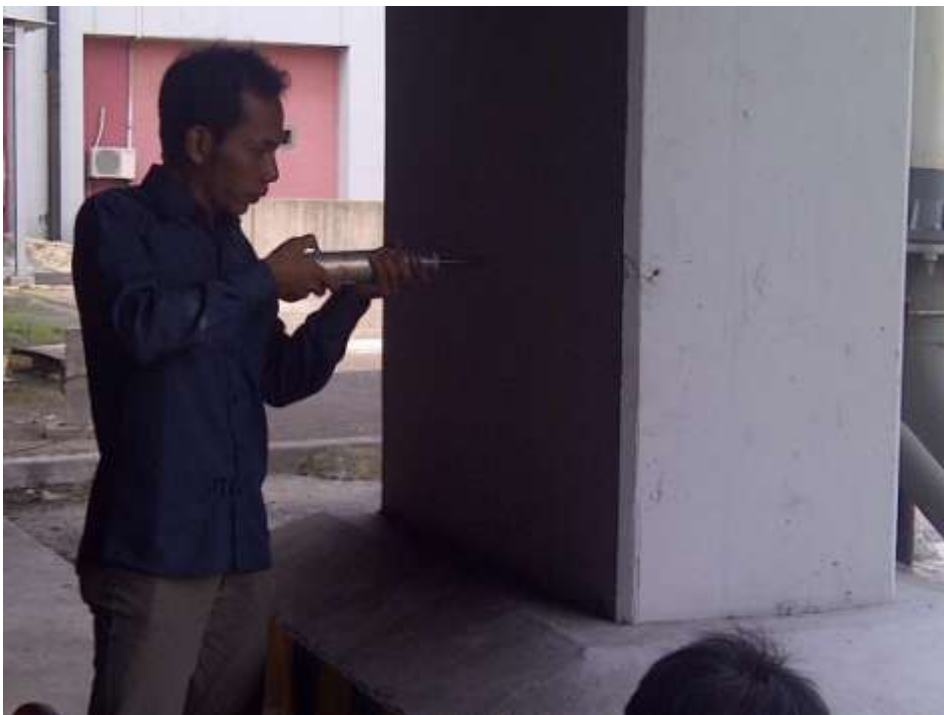
M. UJI HAMMER TEST TERMINAL 1C SHOPPING ARCADE SEBELAH KANAN AREA BREAKDOWN
