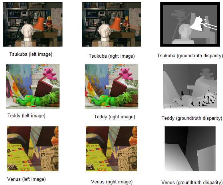
Fig. 2. Tsukuba, Teddy and Venus stereo images: Left image, right Image and ground truth
