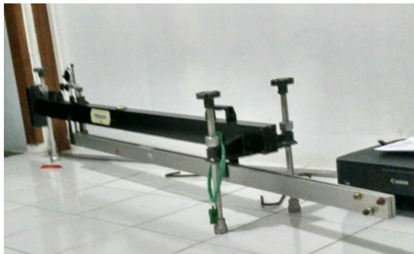
Alat uji Benkelman Beam
