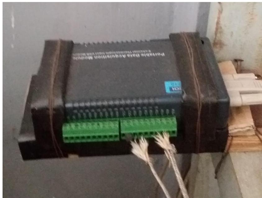
Gambar 3.9 Advantech USB-4718 Portable Data Acquisition Module
