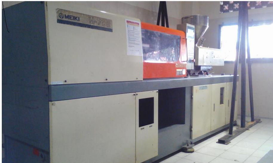
**Gambar 3.4** Mesin *injection molding* meiki 70B
