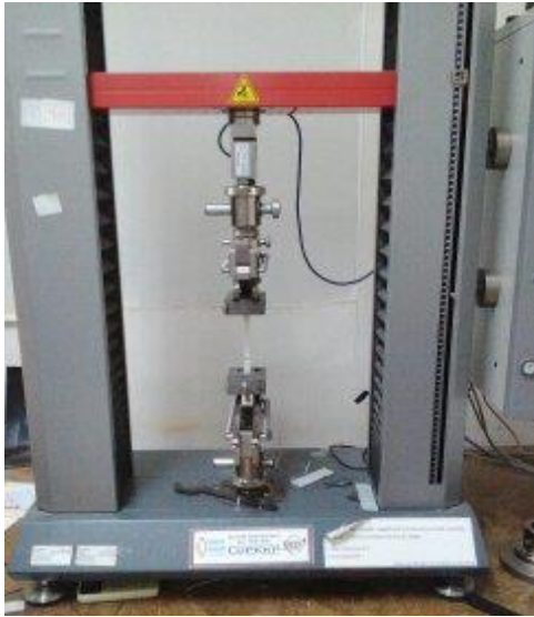
Gambar 2.2 Alat uji kuat tarik Zwick roell (germany).
