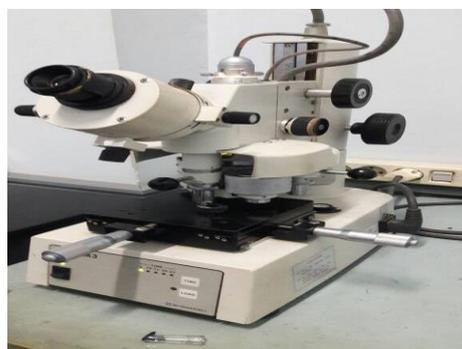
Gambar 3.12 Alat Uji Kekerasan Vickers
