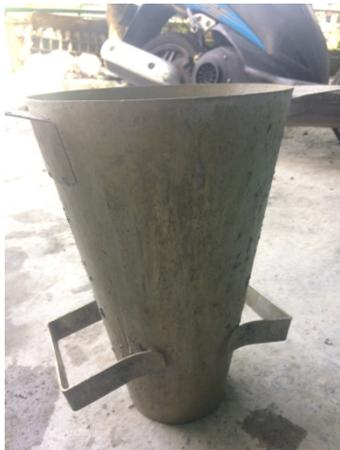
Gambar 4.7 Kerucut Abrams
