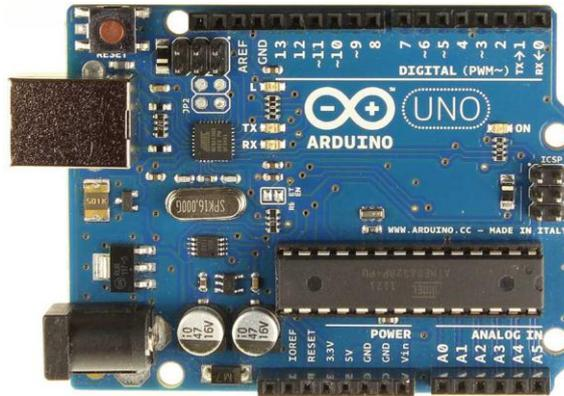
Gambar 2. 4 Board Arduino UNO R3
