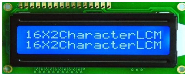
Gambar 2. 5 LCD 2 X 16
