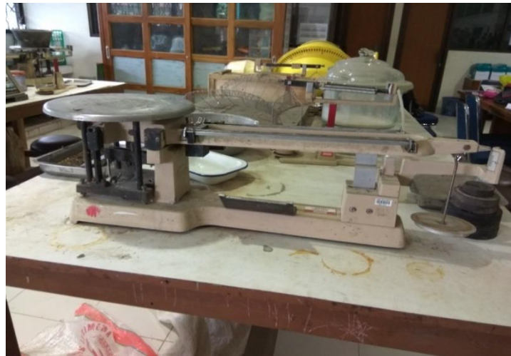
Gambar 4.2 Timbangan ( neraca ohaus )
