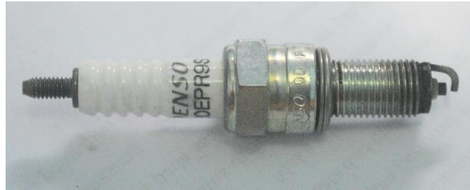
Gambar 3.8 Busi Standar DENSO U20EPR9
