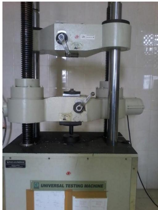
Gambar 2.12 *Universal Testing Machine* (*UTM*)
