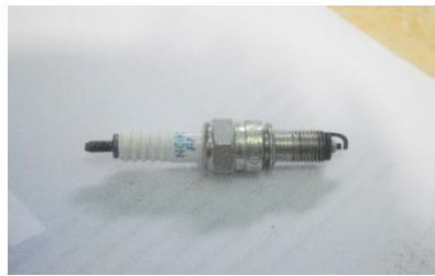
Gambar 2.13 Jenis busi Resistor
