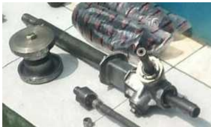
Gambar 4.13 Sistem kemudi rack and pinion
