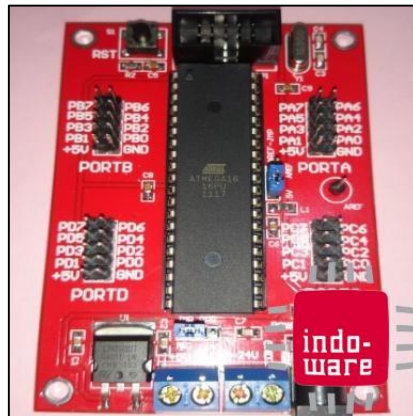
Gambar 3.14 Kontroler motor stepper ATMEGA16 Model A ( www.indo-ware.com/mikrocontrol )
