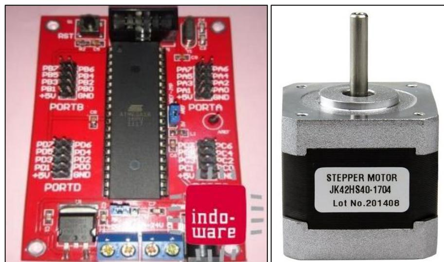
Gambar 4.24. *Nema 17 stepper motor single axis Controller.*
