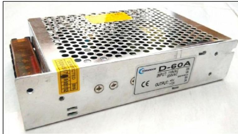
Gambar 4.23. *Power supply* kontroler ECM *single axis* .
