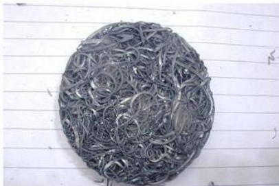
Gambar 7. Bilet Geram Besi ( \text{Fe}_2\text{O}_3 )
