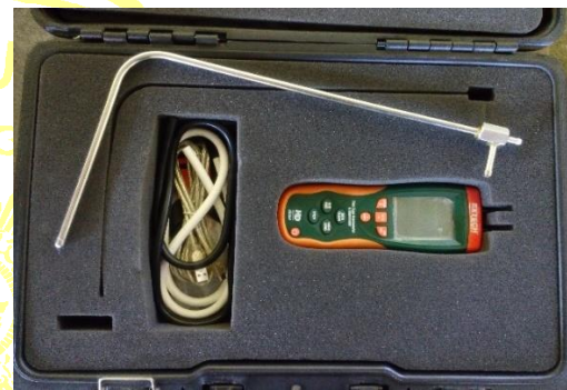
Gambar 9. Extech HD350 Pitot Tube Anemometer & Manometer
