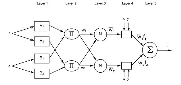
Figure 2: The typical architecture of the ANFIS
