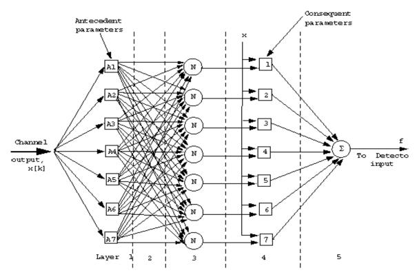
Figure 4: The Adaptive Neuro Fuzzy Inference System (ANFIS) architecture of the research
