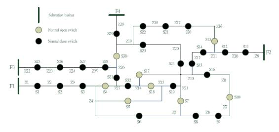
Figure 5: The IEEE standard distribution network before reconfiguration under study
