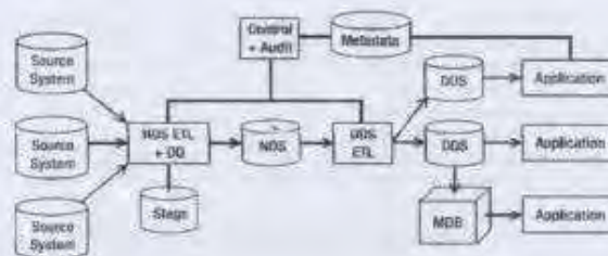
Gambar 1. NDS + DDS data flow architecture
