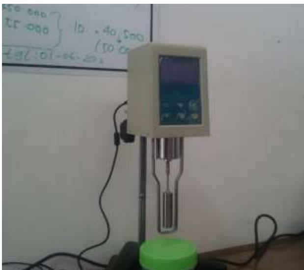
Gambar 3.5 Viskometer
