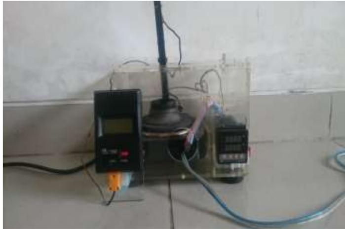
Gambar 3.7 Alat Uji *Flash Point*
