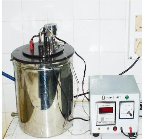
Gambar 2.2 Kalorimeter Bomb (Rahardi 2017)
