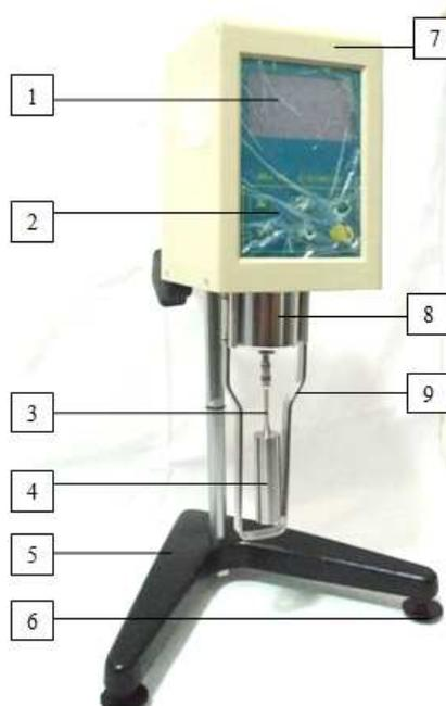
Gambar 3.18. *Viscometer* NDJ 8S
