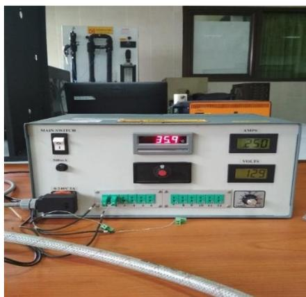
**Gambar 3.4.** *Thermal Conductivity of Liquid and Gases Unit*
