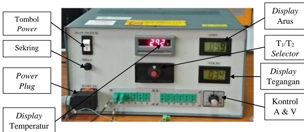
**Gambar 3.12.** Bagian-bagian *Heat Transfer Unit*
