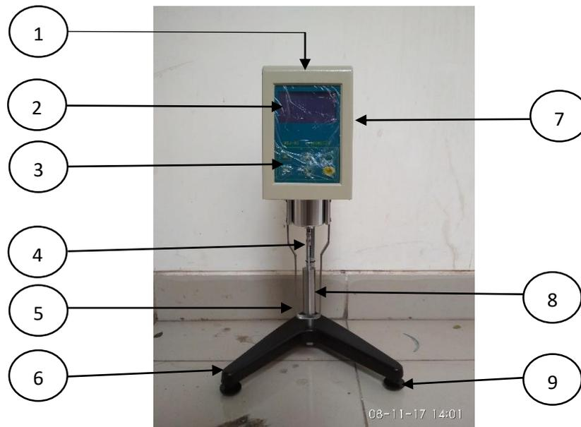
**Gambar 3.20.** Bagian-bagian Viskometer NDJ 8S
