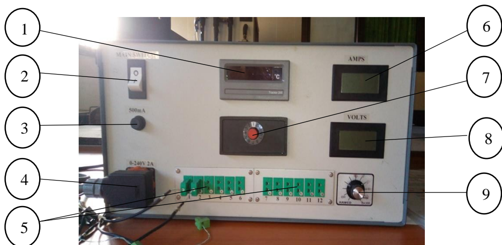
Gambar 3.38 bagian-bagian heat transfer unit
