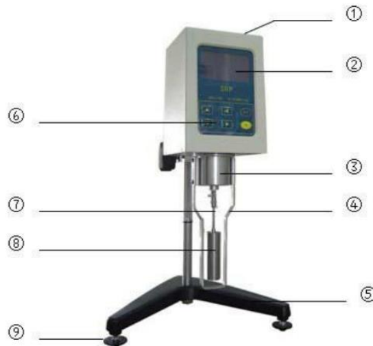
Gambar 3.21 Bagian-bagian viskometer NDJ 8S (Sumber : Manual book)
