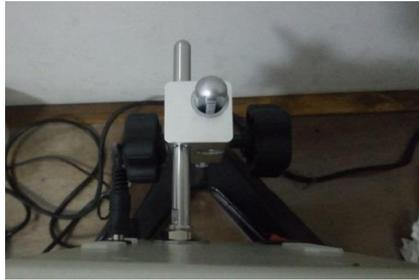
**Gambar 3.17** Stik support viscometer
