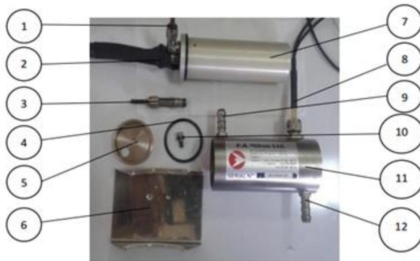
**Gambar 3.32** Bagian-bagian *Heater*
