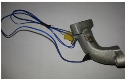
**Gambar 3.34** *Manifold intake* telah dipasang sensor termocouple
