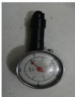
**Gambar 3.59** Tire pressure Gauge
