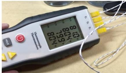
**Gambar 3.12** Termopcouple thermometer HT-9815
