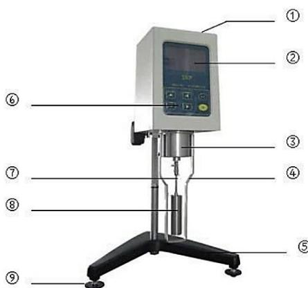
**Gambar 3.14** Bagian-bagian *Viscometer* NDJ 8S
